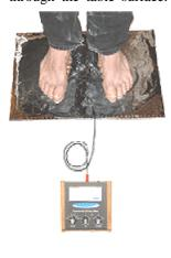
measurements, and place some insulating cardboard or other material underneath the wood base of the Small Plate Electrode.
